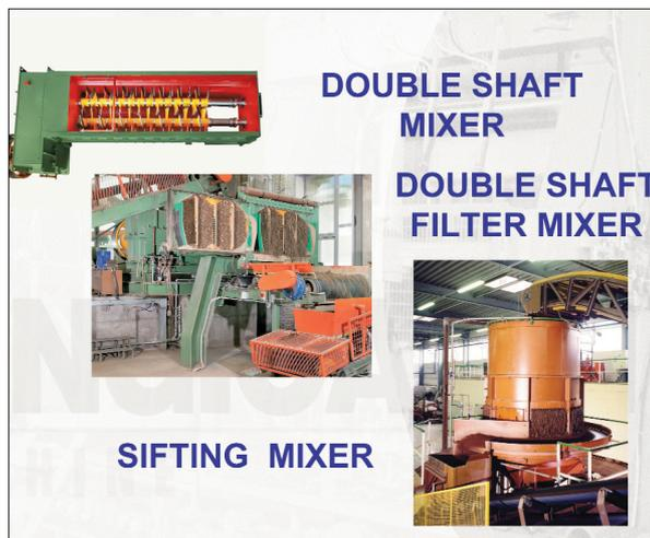
Fig. 4 "Mixers" which can be the traditional double shaft or the vertical sifting mixer
