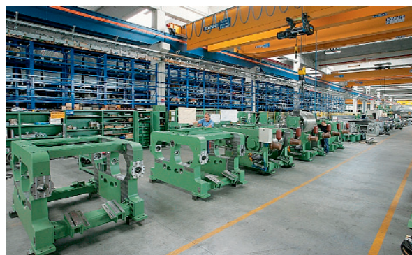
Fig. 3 Bongioanni Macchine's premises: assembly line of roller mills
