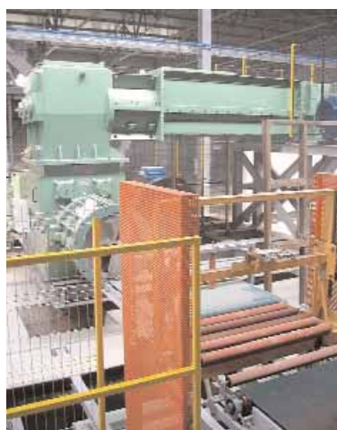
Fig. 3 a-b View of the extruder type TECNO having an auger of 750 mm
