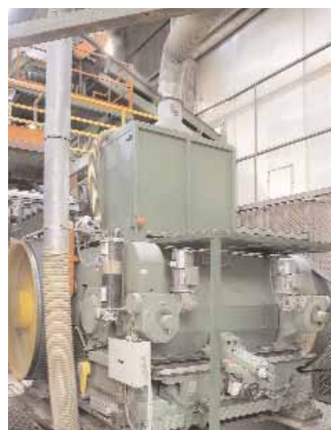
Fig. 3 a-b View of the extruder type TECNO having an auger of 750 mm
