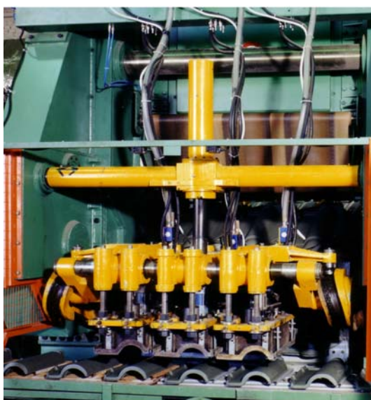
16PV press, detail of fettling unit Pressa 16PV, dettaglio sbavatore
