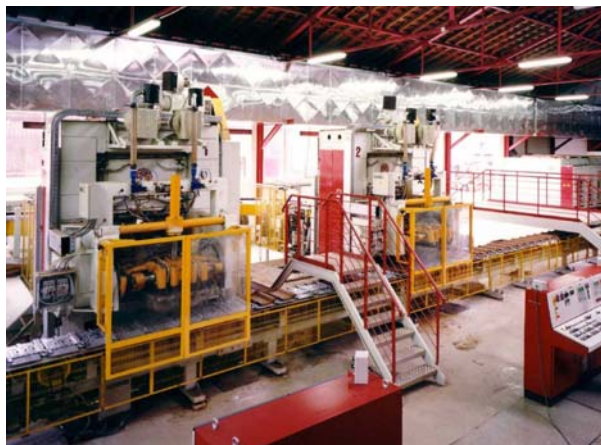
Two 13PV type 2-mould presses • Due presse a 2 stampi tipo 13PV
